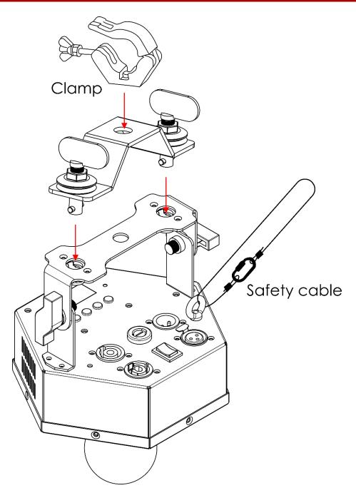
The Edison can be mounted to any kind of truss with quick locks and a clamp.
