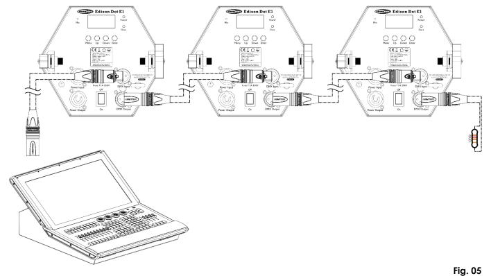
Note: Link all cables before connecting electric power
