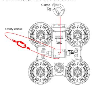
The Stage Blinder 4 LED can be placed on a flat surface or fitted to any kind of truss with a clamp.
