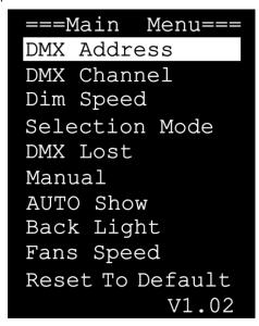
Press the **UP/DOWN** buttons to navigate through the Main Menu. Press the **ENTER** button to open the submenu.
