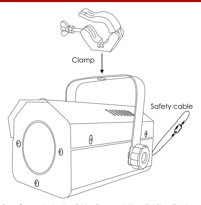
The Bumper Flower can be placed on a flat stage floor or mounted to any kind of truss with a clamp.
