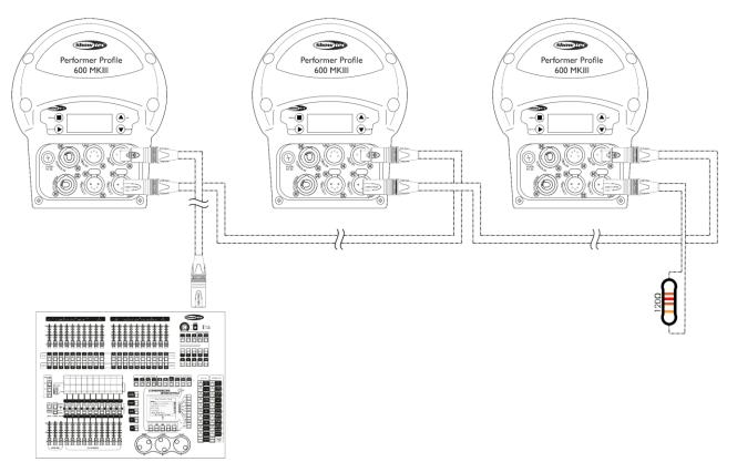
Note: Link all cables before connecting electric power
