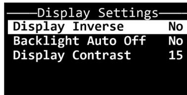
02) Press the **ENTER** button to confirm the selection and open the pop-up submenu where you can adjust the settings.
