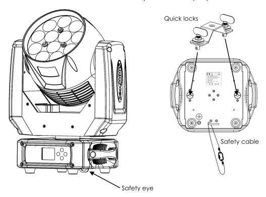
The Phantom can be placed on a flat stage floor or mounted to any kind of truss with quick locks and a clamp.
