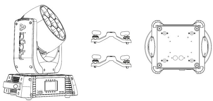
The Infinity can be placed on a flat stage floor or mounted to any kind of truss with a clamp.
