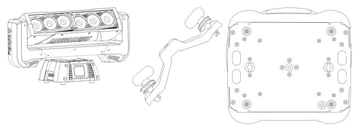
The Infinity can be placed on a flat stage floor or mounted to any kind of truss with a mounting bracket, a clamp and quick-locks.
