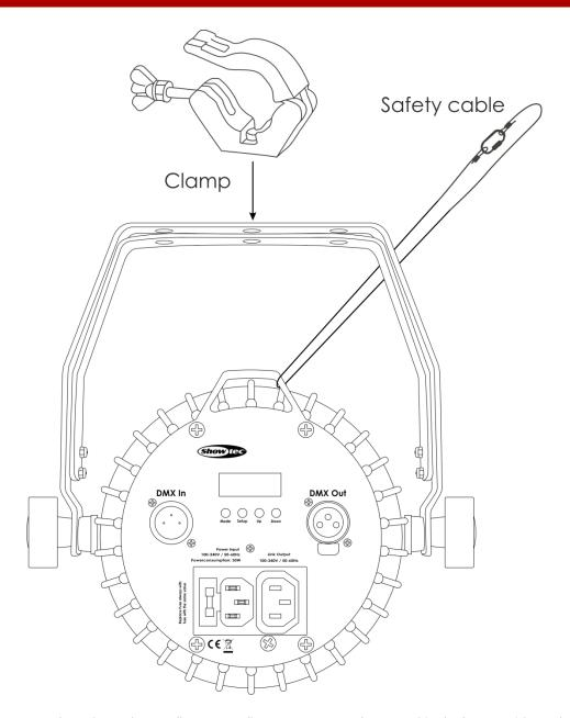
The Power Spot can be placed on a flat stage floor or mounted to any kind of truss with a clamp.
