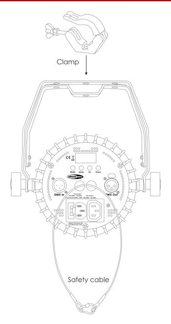
The Power Spot can be placed on a flat stage floor or mounted to any kind of truss with a clamp.
