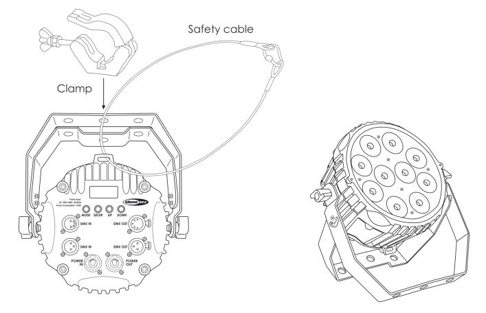
The Powerspot 10 SW can be placed on a flat stage floor or mounted to any kind of truss with a clamp.
