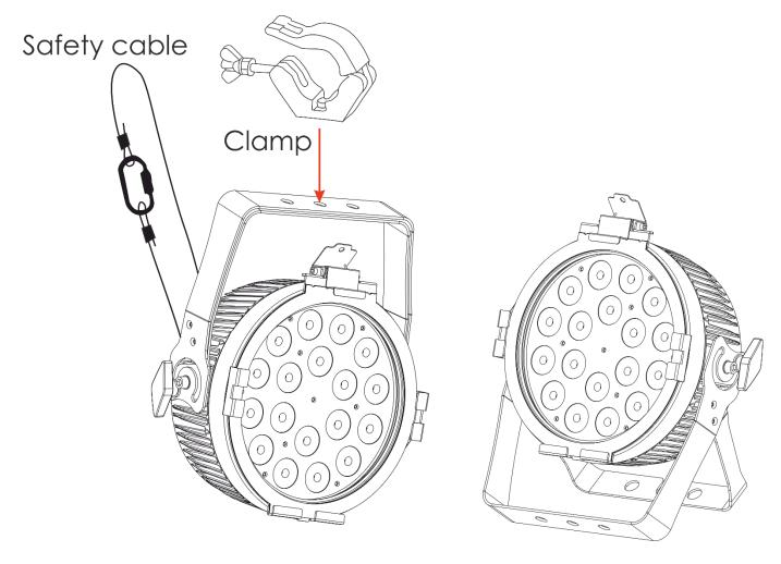
The Compact Par 18 Q4 can be placed on a flat stage floor or mounted to any kind of truss with a clamp.
