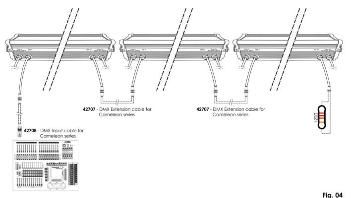
Note: Link all cables before connecting electric power
