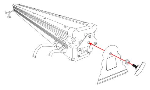
The Cameleon Bar 24/1 UV can be placed on a flat stage floor or be mounted to a wall.
