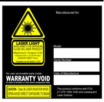
This laser product is a Class IIIB laser and has an Interlocked housing.
