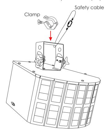
The Double3 Derby LED Q6 can be mounted to any kind of truss with a clamp.
