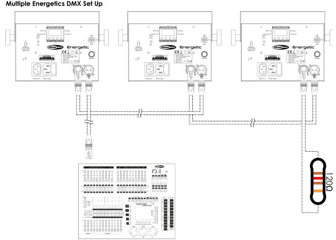
Note: Link all cables before connecting electric power
