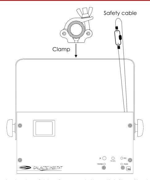
The Galactic can be placed on a flat stage floor or mounted to any kind of truss with a clamp.
