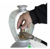
02) Activate the FX Ice Jet one more time to remove the remaining pressure from the hose.
