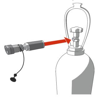
07) Connect the CO<sub>2</sub> hose to the CO<sub>2</sub> bottle-to-hose connector on the new CO<sub>2</sub> cylinder.
