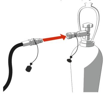
16) Open the CO<sub>2</sub> cylinder and check for leaks. If the gas hose is **not properly** connected, **gas can escape**. If this is the case, turn the couplings tighter until gas is no longer escaping.
