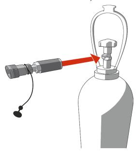
15) Connect the  $CO_2$  hose to the  $CO_2$  bottle-to-hose connector on the  $CO_2$  cylinder. Turning it by hand should suffice! Use the wrench only if the coupling continues to leak.
