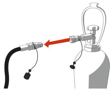
05) Remove the CO<sub>2</sub> bottle-to-hose connector from the cylinder.
