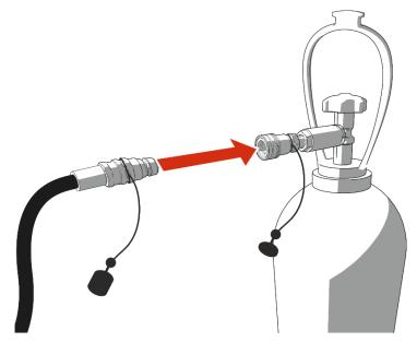
08) Move the manual CO<sub>2</sub> valve back to the CLOSED position.
