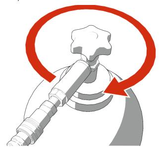
03) Move the manual CO<sub>2</sub> valve to the OPEN position to release the pressure from the system.
