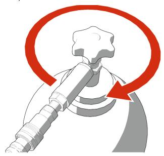
07) Move the manual CO<sub>2</sub> valve to the OPEN position, to release the pressure from the system.
