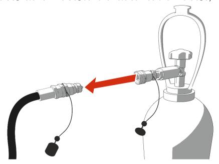
10) Remove the CO<sub>2</sub> bottle-to-hose connector from the cylinder.
