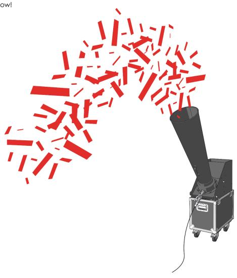
05) When you are finished blasting confetti, move the manual  $CO_2$  valve back to the CLOSED position.
