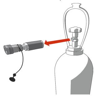
06) Connect the CO<sub>2</sub> bottle-to-hose connector to a new CO<sub>2</sub> cylinder.
