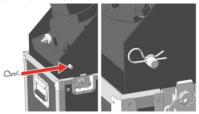
06) Set the angle of the woofer by aligning the back pinhole with one of the four predefined holes in the case.
