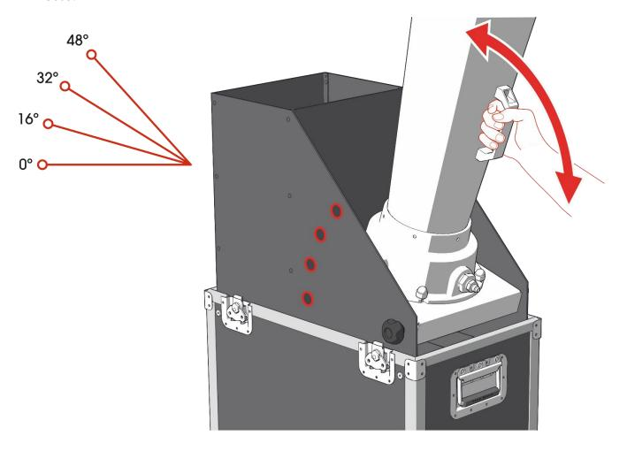
07) Insert the second pin through the back pinholes to secure the position of the woofer.
