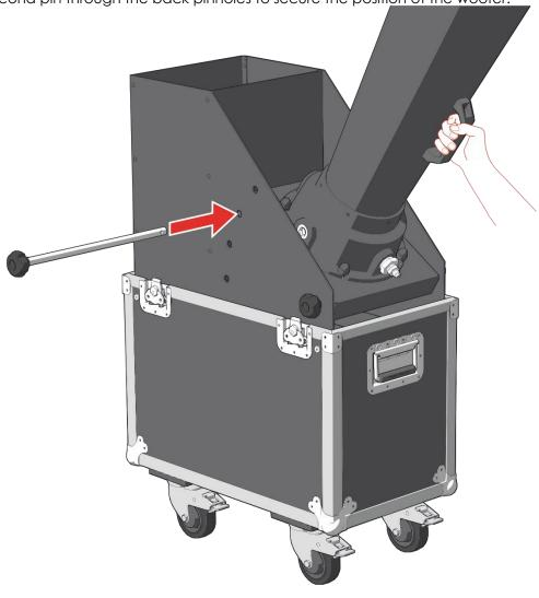
08) Secure the pin with a safety split pin.
