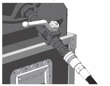
02) Close the connected CO<sub>2</sub> cylinder.
