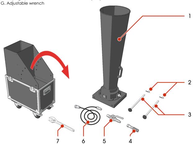
04) Place and hold the woofer in the case and insert a pin through the front pinholes. Make sure that the  $CO_2$  input of the woofer is positioned at the front.
