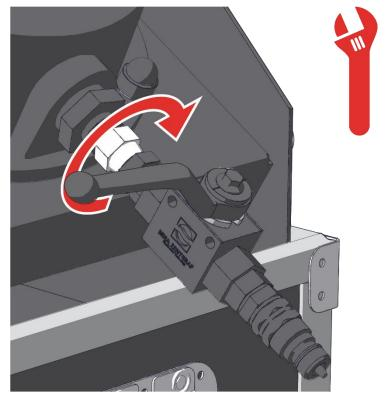
12) Connect the CO<sub>2</sub> hose to the CO<sub>2</sub> valve.
