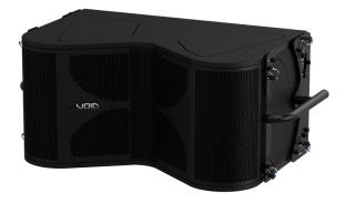
Specially designed to extend the low frequency range of the Arcline line array, the Arcline 212 features two 12" 900 W low frequency drivers. This makes it possible to extend the frequency response range to as low as 55 Hz, while also reaching up to 120 Hz.
