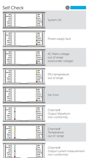
1. An 8  $\Omega$  dummy load is needed to measure the output current. If the dummy load is not applied the system reports a fault.
