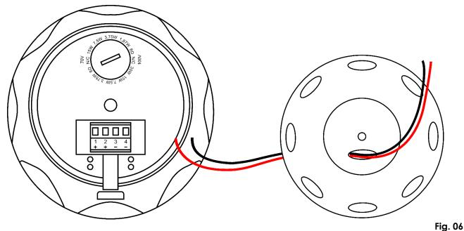
02) Connect the speaker cables to the device (Fig. 07). See **4.5**. **Connecting to Amplifier** on pages 12–14 for more information.
