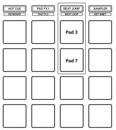
Pad 3 on the left lit: When rekordbox is running, controller operation depends on the rekordbox dj functions. When rekordbox is not running, the unit operates as a general MIDI controller. (default)
