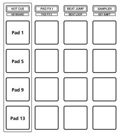
Pad 1 on the left lit: Demo mode off (default) Pad 5 on the left lit: 1 minute Pad 9 on the left lit: 5 minutes Pad 13 on the left lit: 10 minutes
