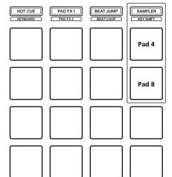
Pad 4 on the left lit: The MIDI (control change) value rises when sliding the touch strip toward the maximum level. (default) Pad 8 on the left lit: The MIDI (control change) value rises when sliding the touch strip toward the minimum level.
