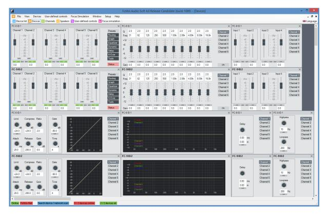
At the same time, **Fohhn Audio Soft** also enables the management and control of up to 254 active **Fohhn** devices, giving you constant feedback on both the status of the connected devices and their respective parameter values.
