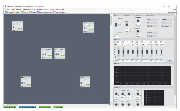
Please note that, with devices belonging to the **Xperience-Series**, passively connected subwoofers will not show up in the *Speakers* view – only the two output channels of the relevant device(s). In most cases it is probably easier to control these particular devices using the *Devices* view.
