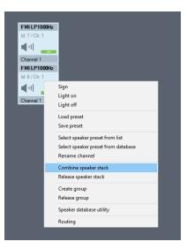
In the loudspeaker pictograms, next to the ID, an S will appear: These means that the loudspeakers are now "stacked".
