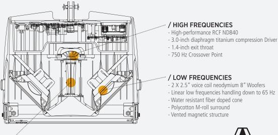
The custom 4 PATH-designed waveguide allows precise coverage of  $100 \times 15$  degrees, while also delivering an excellent, linear high-frequency response. The unique shape of the four ducts forming the guide creates an ideal isophasic load from 750 Hz to the highest audible frequencies.
