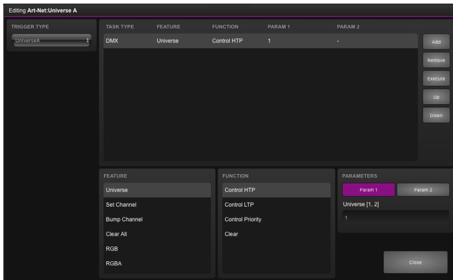
Figure 10.5: Converting Art-Net to DMX step 2
