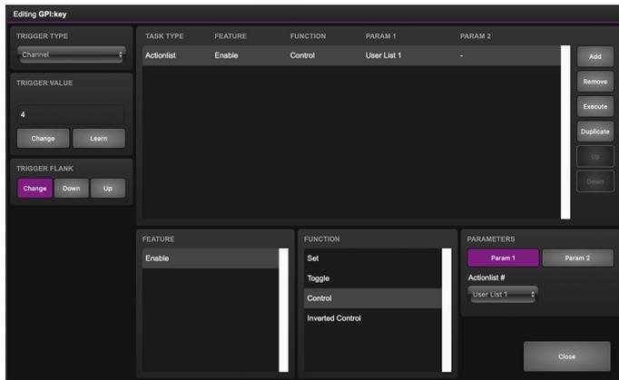
For brevity the state of the GPI port 4 is ignored at start-up. Usually additional actions are created to *Refresh* this port on start-up.
