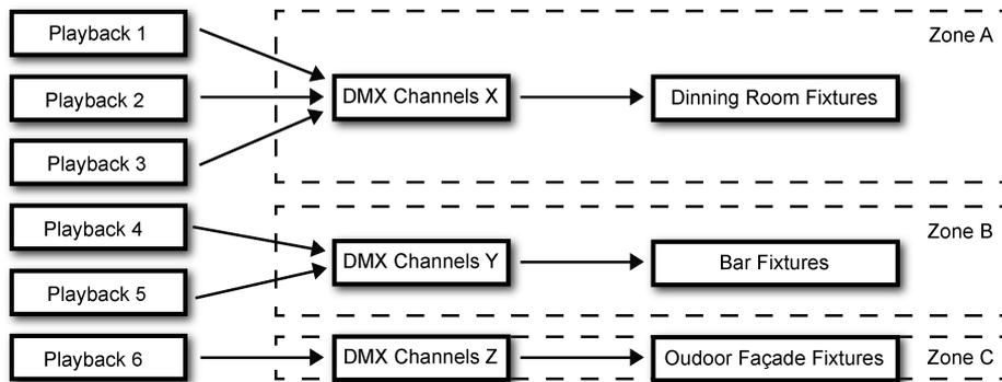
Figure 8.3: Playbacks controlling zones in a restaurant
