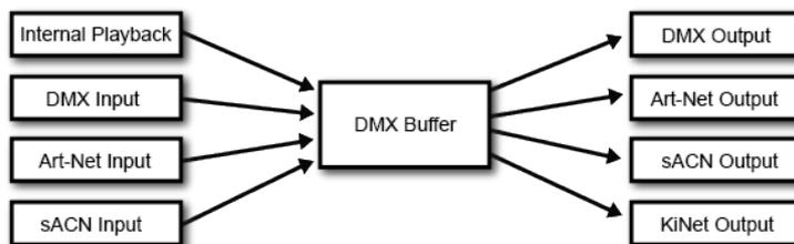
Figure 10.3: DMX merging data flow
