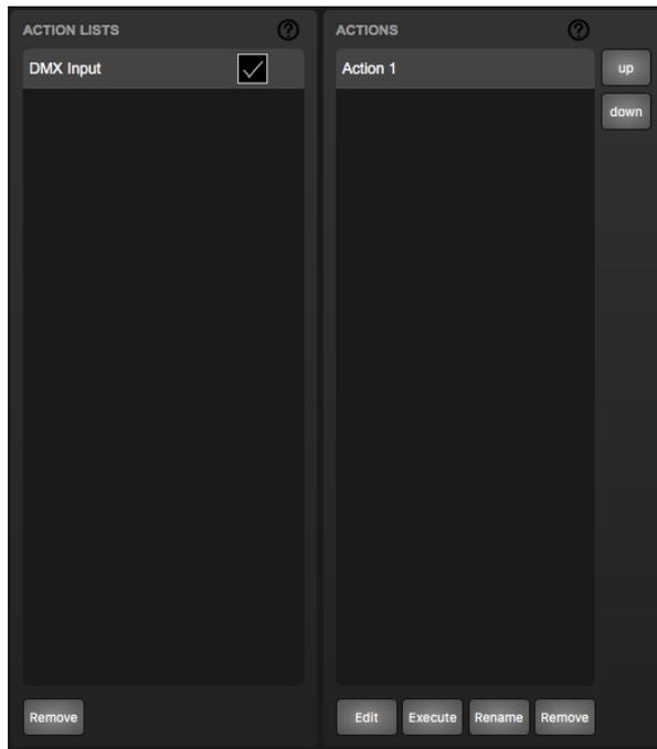
Edit the action. Set the *Trigger Type* to *UniverseA*. Add a *DMX* task and set its feature to *Universe* and its function to *Control HTP*, the first parameter should be set to 1.
