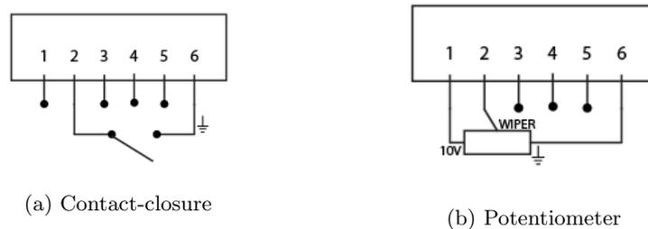
Figure 2.3: GPI Wiring examples
