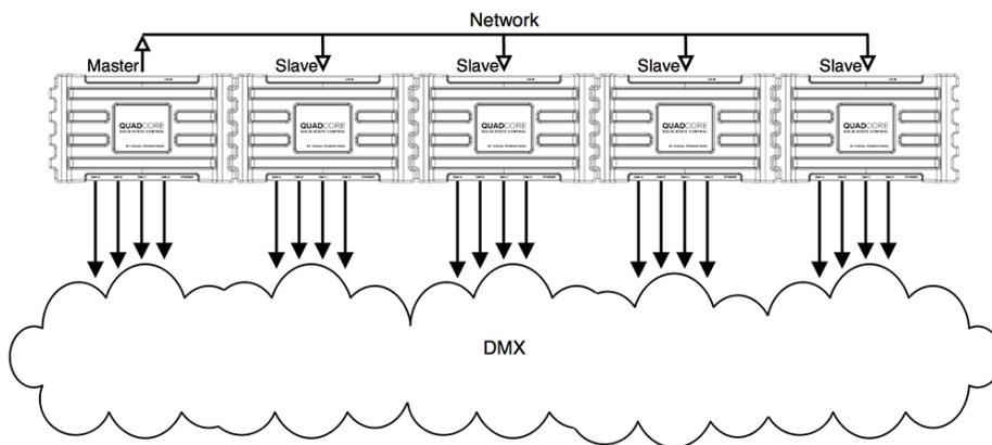
Figure 6.3: Master/Slave setup
