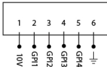
Figure 2.2: GPI Pinout
