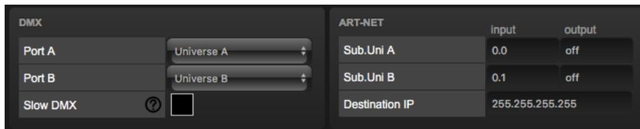
Figure 10.6: Converting Art-Net to DMX step 3
