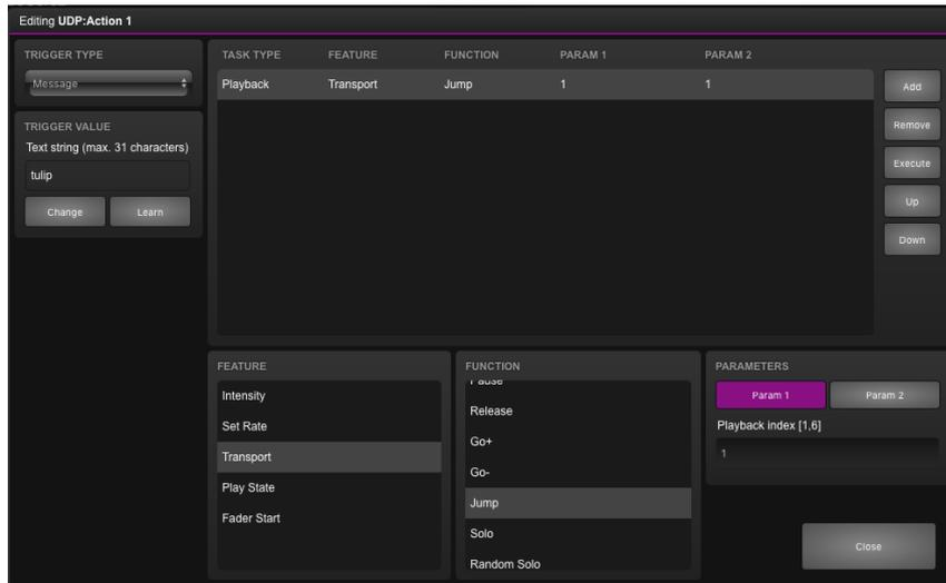
Press the 'Close' button, select the second action and press 'Edit' again. Change this trigger value to "crocus". Add a task by pressing 'Add' and choose the 'Playback' task-type. Select the newly added task and set the 'feature' to 'Transport' and set the 'function' to 'Jump'. Parameter 1 should be set to '1' (addressing the first playback) and parameter 2 should be set to '2' (jump to the second cue).
