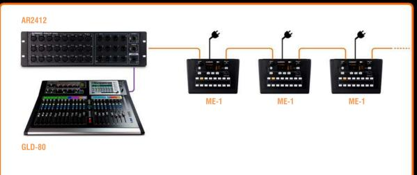
ME-1 can be connected to the Monitor port on the AR2412 or any other available dSNAKE or Expander port in a GLD system. Channel names and stereo linking are picked up automatically from the digital stream.
