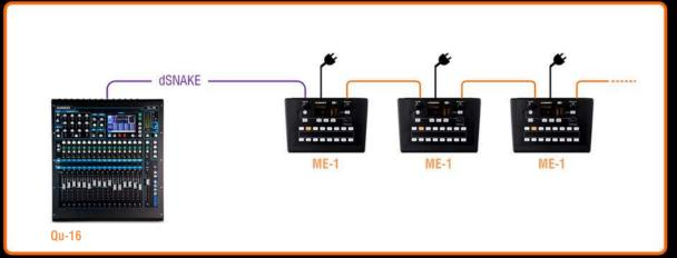
ME-1 can be connected to the dSNAKE port on a Qu mixer or to an Expander port on an dSNAKE AudioRack. Channel names and stereo linking are picked up automatically from the digital stream.
