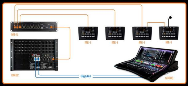
ME-1 can be connected directly to the dedicated ME port on a dLive DM MixRack, or via a ME-U hub. Channel names are picked up automatically from the digital stream.
