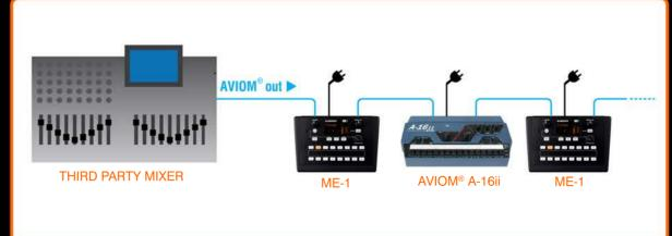
ME-1 can integrate with other professional mixers via Dante, EtherSound or MADI thanks to the ME-U hub (see previous page), or interface directly with existing AVIOM® systems. When connected to an AVIOM® A-Net® Pro16® device, ME-1 seamlessly detects the AVIOM® stream and switches automatically to AVIOM® compatibility mode, limiting the number of sources to 16.
