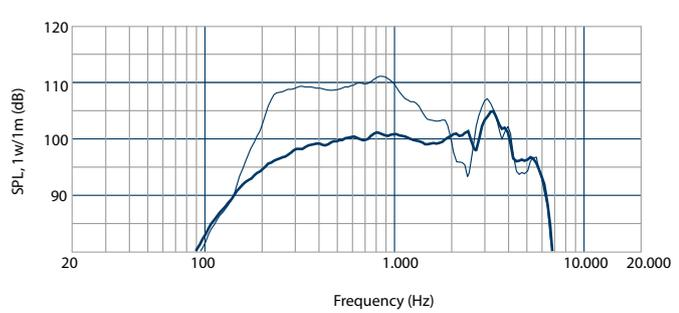
Frequency response curve of the loudspeaker taken in a hemispherical, free field environment and mounted on IEC panel (ticker curve) and on a 60x40 horn (lighter curve)
