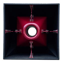
As part of the Nexus low frequency system, the Nexus Q delivers impressive upper bass frequencies via a new enclosure design. The four high power 12" drivers use a front-loaded horn to achieve high efficiency and a rear port with a newly developed pressure gradient arrangement. This configuration results in unparalleled output, definition, and total elimination of colouration from any turbulent or mechanical port noise.
