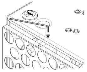
Figure 6.4: Bolt removal
