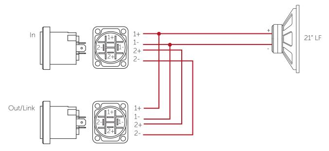
Figure 5.2: Wiring diagram
