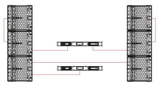
Figure 5.8: 6 x Nexus XL: 8  $\Omega$  per channel/2 amplifier
