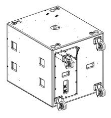
Figure 6.2: Wheel removal
