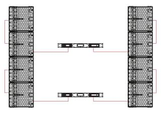
Figure 5.9: 8 x Nexus XL: 4  $\Omega$  per channel/2 amplifier
