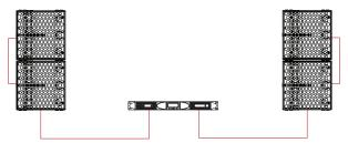
Figure 5.7: 4 x Nexus XL: 4  $\Omega$  per channel/1 amplifier
