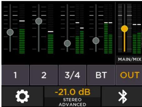
To change the value of any fader on this page, touch the fader once and use the encoder to modify its current value; the encoder highlights in yellow and the current value is shown in yellow above the encoder itself.
