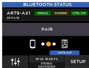
*Note: go to SETTINGS > SYSTEM SETTINGS > UTILITIES > DISPLAY to modify Timeout to Idle and Time to Home Page values, both in seconds.*
