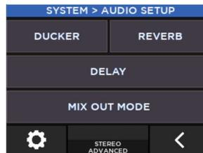
The **DUCKER** page contain individual enable buttons to allow level reduction of destinations (ch. 2, ch. 3-4 or BT) when a signal is present on ch. 1 or ch. 2.
