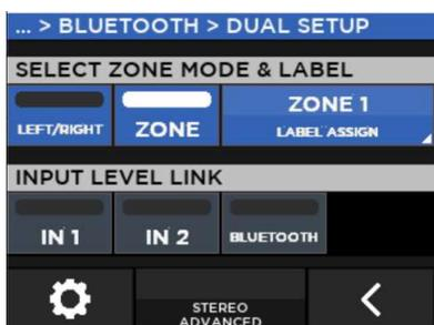
The DUAL system is set in ZONE mode; Bluetooth audio is summed to mono and sent to both speakers. MAIN output levels are independent.
