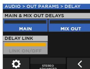
Maximum delay value is 136 ms, corresponding to 46.6 meters.
