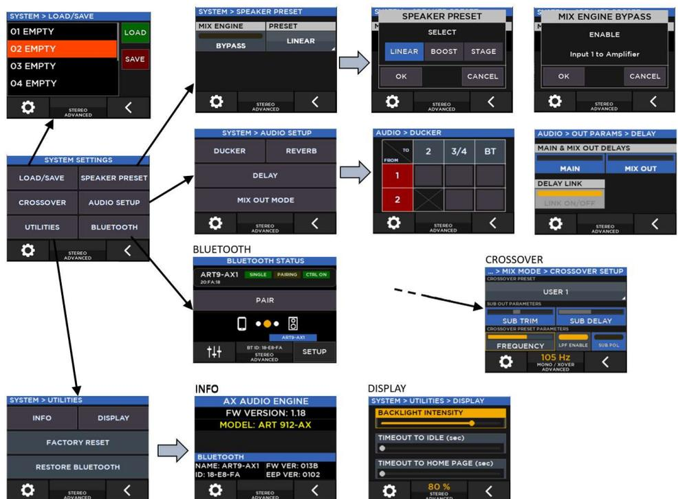
The **LOAD/SAVE** page allows saving and recalling the full configuration of the unit, with the exception of:
