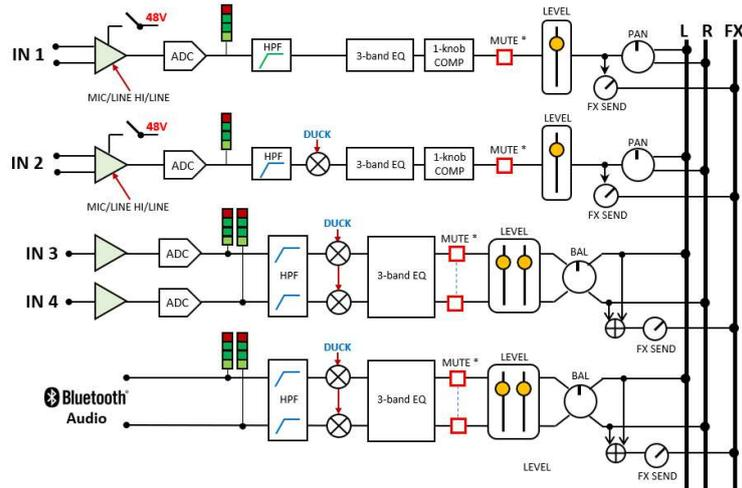
Inputs 1 and 2 feature a Compressor section, and can be set as a stereo pair or independent; inputs 3-4 and BT are always managed as a stereo pair, and do not feature the Compressor section.
