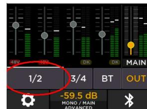
Please note that 48V on/off control is enabled only when input PRE is set to MIC.
