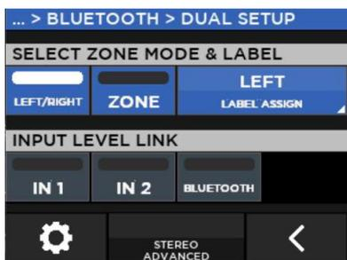
The DUAL system is set in LEFT/RIGHT mode; Bluetooth audio is running in stereo (one channel per speaker), and MAIN output level of the speakers are linked.
