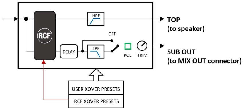
Internal, read-only presets have been created assuming specific subwoofer configurations; please follow the table below to correctly configure the subwoofer unit connected to MIX OUT.
