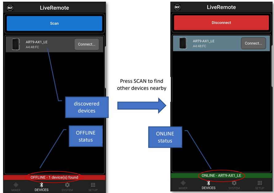
For audio connection, the ART 9-AX behaves like a usual Bluetooth speaker: press PAIR on the unit (available on the main Bluetooth page), then open the Bluetooth settings on your smartphone and select the ART 9-AX speaker. Take care in avoiding selecting entries with \_LE suffix, as they are not available for audio streaming.
