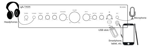
**Note!** Turn the Volume Regulator to MIN (max counter clockwise) before connecting or disconnecting any additional device.
