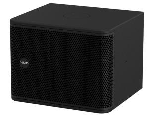
The Venu 112 V2 is a single 12" compact low frequency enclosure, providing a frequency response of 40Hz – 160kHz  $\pm 3$  dB and efficiency of 99dB1w/1m. Features include a tough 12" high excursion transducer with a 4" voice coil and a strong enclosure made entirely from 15 mm multi-laminate birch plywood.
