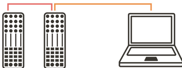
K1 + K2 CONTROLLERS via X:LINK + LAPTOP via USB
