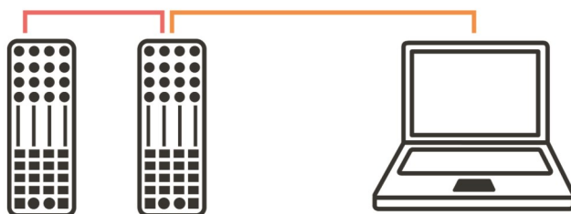
K1 CONTROLLERS via X:LINK + LAPTOP via USB
